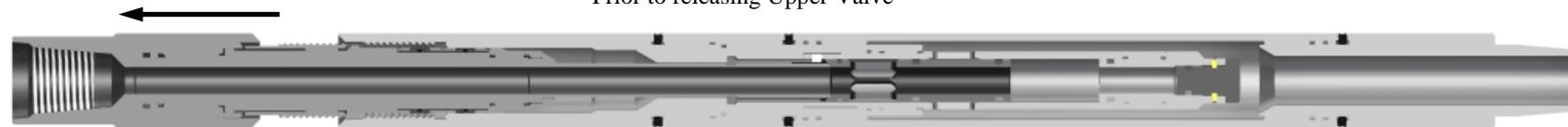
Begin Release Movement – Stinger Assy & Valve Moves Upward. Lower Collet Fingers Expand Into Connector.
