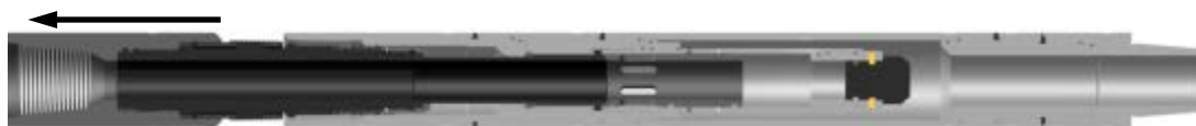
Begin Release Movement – Stinger Assy & Valve Moves Upward. Lower Collet Fingers Expand Into Connector.
