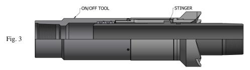
Pin the overshot to the stinger in the tension position (Fig. 3). Run in the tool to the desired depth. Pick up and set down holding right-hand torque. Release the torque once the tool begins its setting procedure. Once the ASI-X is completely set, straight pull to shear the pin and rotate to the left to release the overshot from the stinger.
