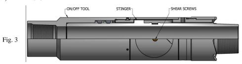
Pin the overshot to the stinger in the tension position (Fig. 3). Run in the tool to the desired depth. Pick up and set down holding right-hand torque. Release the torque once the tool begins its setting procedure. Once the ASI-X is completely set, straight pull to shear the pin and rotate to the left to release the overshot from the stinger.
