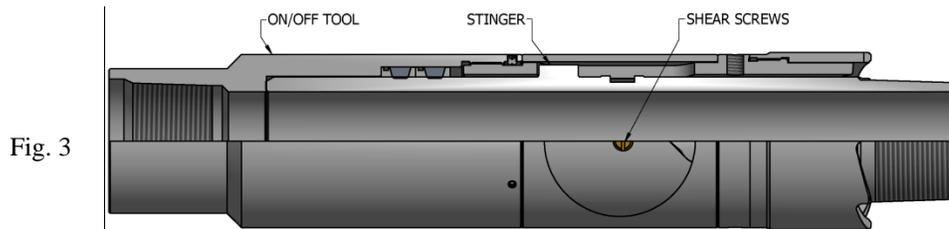
Pin the overshoot to the stinger in the tension position (Fig. 3). Run in the tool to the desired depth. Pick up and set down holding right-hand torque. Release the torque once the tool begins its setting procedure. Once the ASI-X is completely set, straight pull to shear the pin and rotate to the left to release the overshoot from the stinger.
